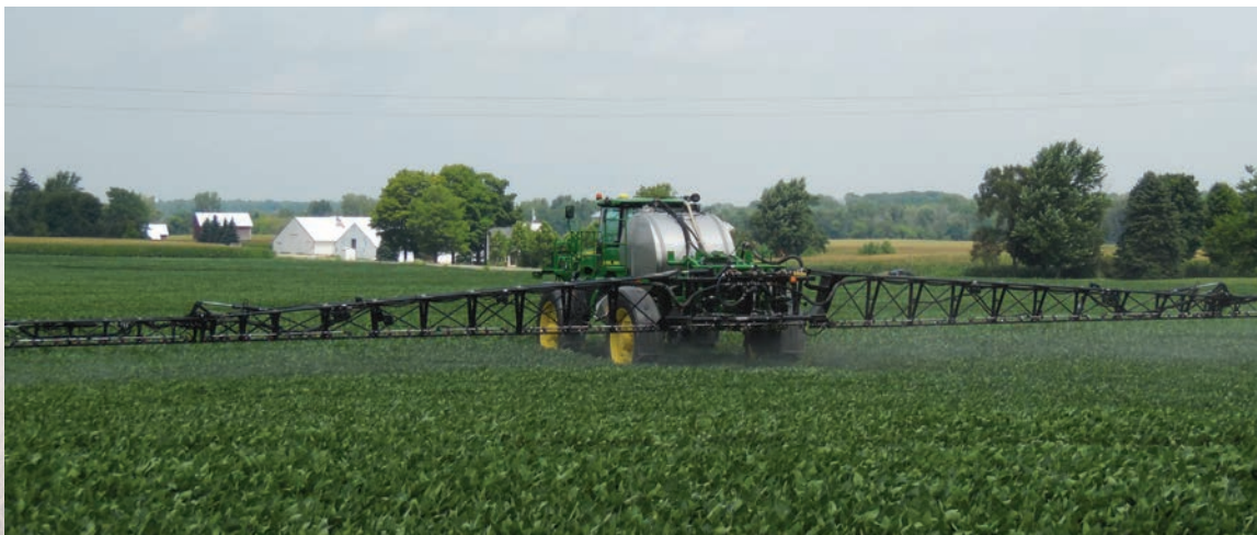
Self-propelled sprayer equipped with a 120 foot boom
